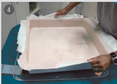
4 Demold after resin cures
