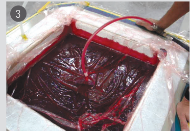
3 Inject room temperature curing infusion grade resin
