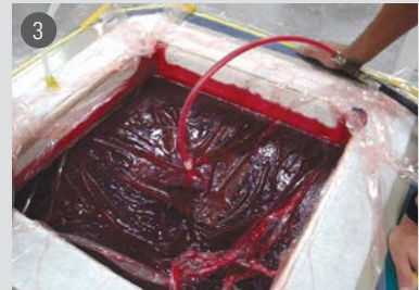
3 Inject room temperature curing infusion grade resin
