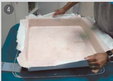
4 Demold after resin cures
