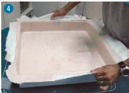
4 Demold after resin cures
