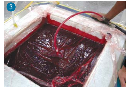
3 Inject room temperature curing infusion grade resin
