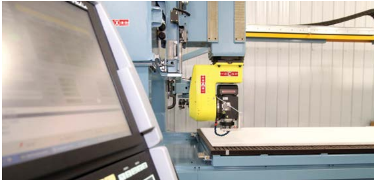
Sheet sizes up to 60" x 240" are possible on Plascore CNC routers.
