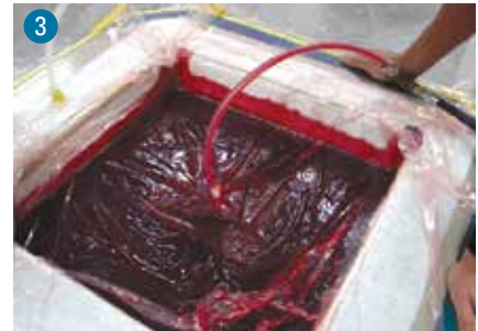
3 Inject room temperature curing infusion grade resin
