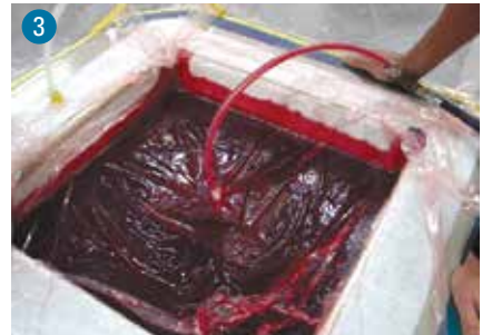
3 Inject room temperature curing infusion grade resin
