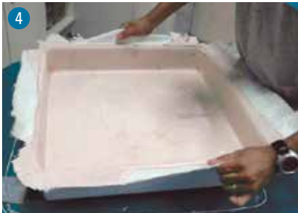
4 Demold after resin cures
