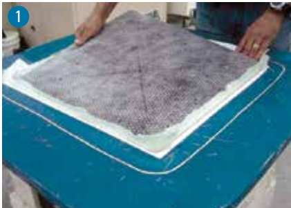
1 Install reinforcements and Infusion Grade PP Honeycomb
