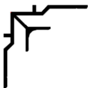
J110 1/4" Liner, Inside Corner
