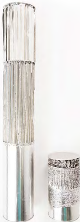
Before and after crushlite and AlTuCore assembly crushing
