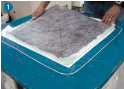
1 Install reinforcements and Infusion Grade PP Honeycomb
