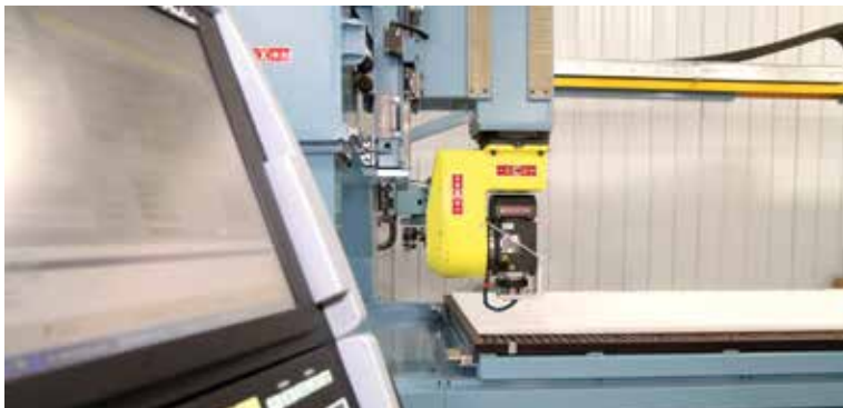
Sheet sizes up to 60" x 240" are possible on Plascore CNC routers.
